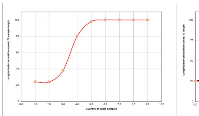
Figure 1. Flame proliferation dependent on cables arrangement.
